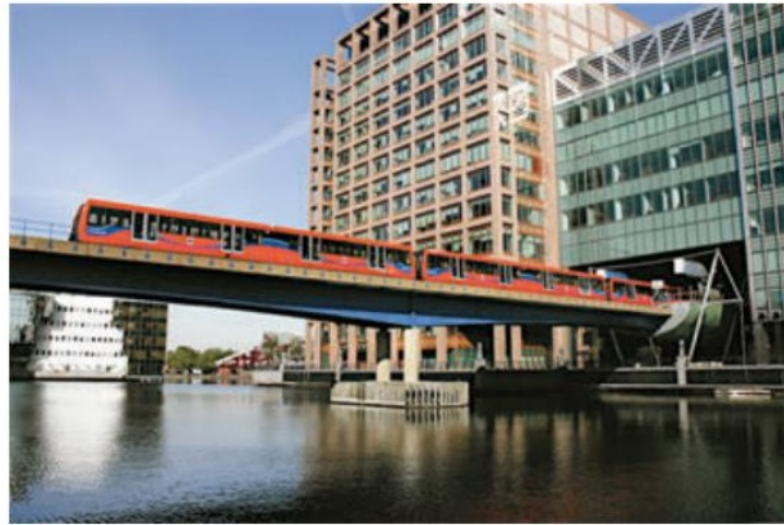
4.80 Trains on the Docklands Light Rail in London, UK, operate without drivers, relying instead on a central, automated control system.
