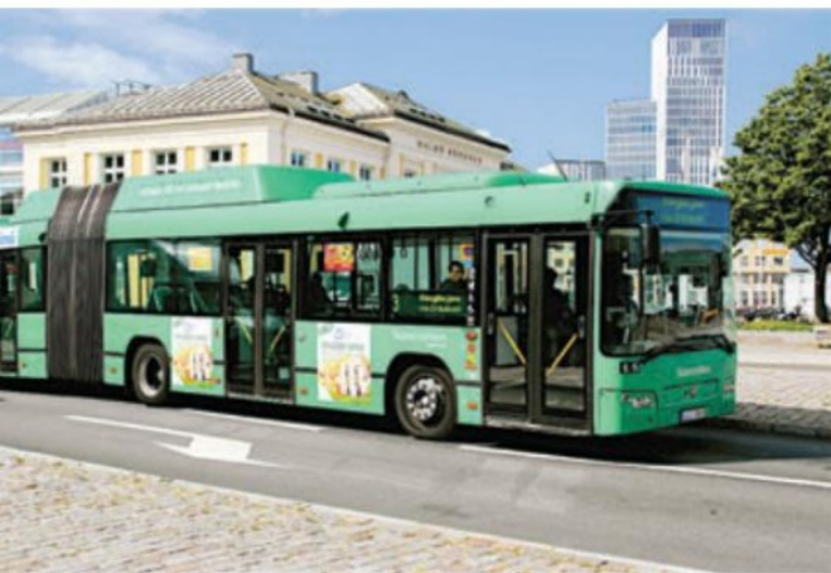
4.48 This bus in central Malmö is powered entirely by biogas that has been produced through recycling food waste.
