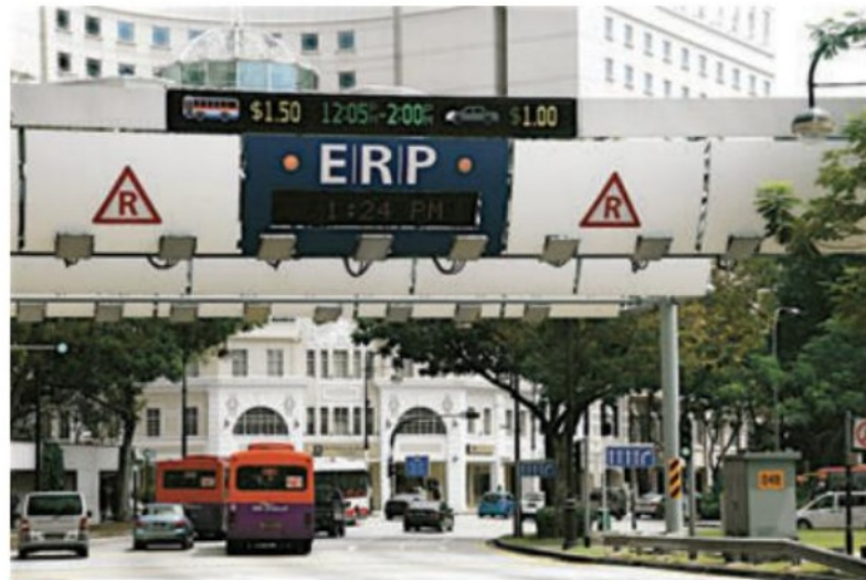
2.24 Electronic road pricing (ERP) is used in many cities (including Singapore, shown here) to regulate the number of cars in the CBD. The toll charged varies according to the type of vehicle and the time of day.
