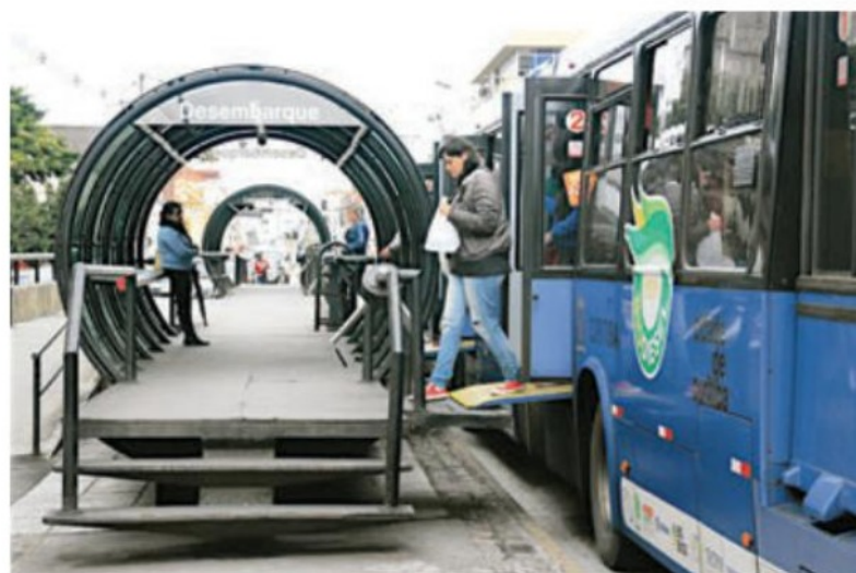
3.46 Boarding ramps snap into place when buses stop at tube stations, facilitating boarding and disembarking.
