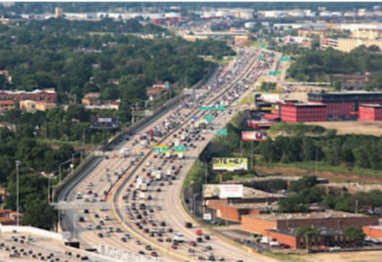
3.34 Road widening and expressway construction can relieve traffic congestion in the short-term, but the extra traffic volume that these roads attract soon leads to further congestion, as seen here on the I-294 freeway in Chicago, Illinois, USA.
